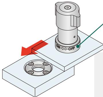
The shank retracts at the OFF position to enable operations without interference with the base plate.
