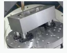
Modular Pull Clamping System enables machining from five sides, resulting in better machining accuracy with a single setup!
