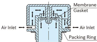
Air comes into the reservoir when the membrane gasket warps owing to vacuum caused by liquid discharge.
