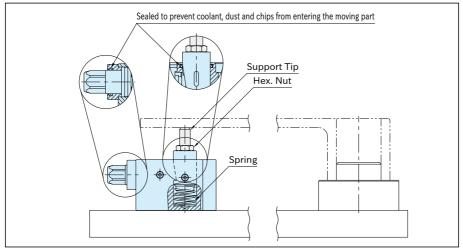
•Load a workpiece, and the piston lowers. Turn the hex. head to lock the piston. •Prevent workpiece vibration and deflection.
