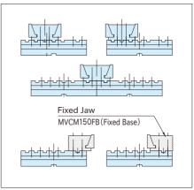
Can attach various fixed jaws at different positions on the base.
