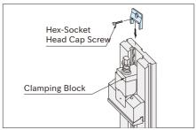
Set the insert in the slot of the base. Prevent slip off of the movable jaw. To hold the insert, use the included hex-socket setscrew as needed.
