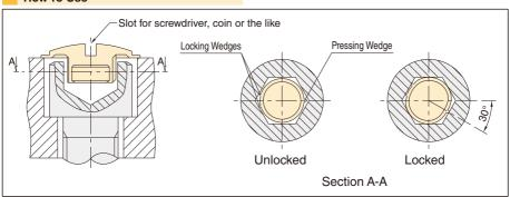
Once a cap is given a 30° turn by using a screwdriver or coin, the 3 wedges on the cyliner are pressed against two flats of the hex socket to generate a strong grip for positive locking. When turned in the opposite direction, the cap gets unlocked for removal.
