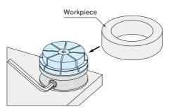
\*) Following the above steps for jaw machining, the clearance between the jaw and the workpiece will be 0.3 mm in diameter.
