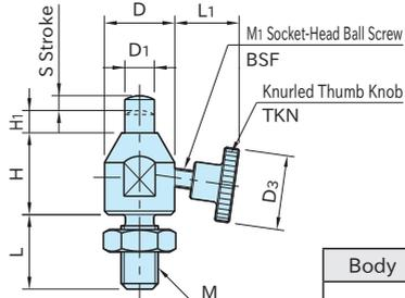
Note: The socket-head ball screw is glued to the knurled thumb knob.
