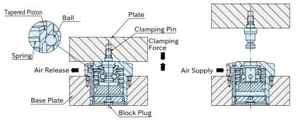
Releasing air allows the spring to push down the tapered piston. The balls pushed by the piston pull down the clamping pin. Keeps clamping without air supply.
