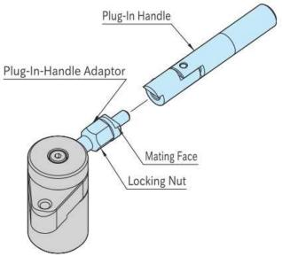
When coupling the handle with the adaptor, ensure that the handle has full contact with the adaptor's mating face. Secure the handle to the adaptor using the lockingscrew if necessary.
