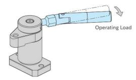
The desired clamping force is reached when the handle folds approximately 15°. See the page of each clamp for the information on operating load vs. clamping force.
