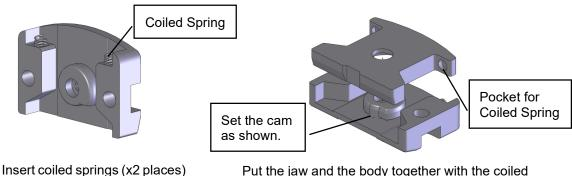
ces) Put the jaw and the body together with the coiled springs staying in the pockets, first on the side of the coiled springs.
