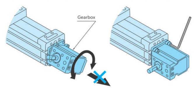
Note: Do not pull the gearbox to the axial direction.
