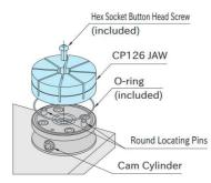
2-2. •Tighten the cam cylinder to clamp the locking ring. (Recommended Tightening Torque:15N·m)
