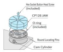
2-2. I lighten the cam cylinder to clamp the locking ring. (Recommended Tightening Torque:15N·m)
