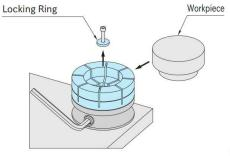
\*) Following the above steps for jaw machining, the clearance between the jaw and the workpiece will be 0.3 mm in diameter.
