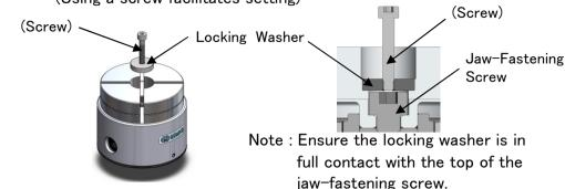
2) Tighten the locking screw to clamp the locking ring.
