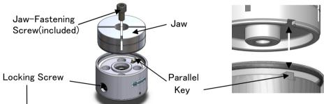
Note: At jaw installation, ensure the locking screw is fully loosened by turning counterclockwise until it stops.
